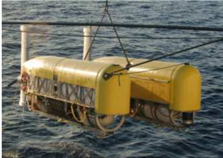
Figure 3.2: The hybrid remotely operated vehicle Nereus configured as an AUV. Photo credit: Louis Whitcomb, JHU.
