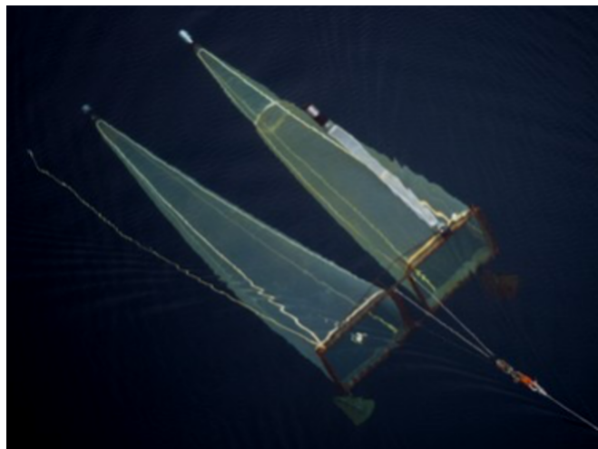
Figure 5. Example of a Double Square Net (DSN) used to sample age-0 fish and mesozooplankton (not the actual DSN lost during the cruise).
