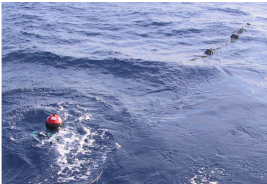
Figure 9. An SVP/OCM drifter just after deployment. The surface ball (bottom left) and drogue (before sinking, top right) are clearly seen.
