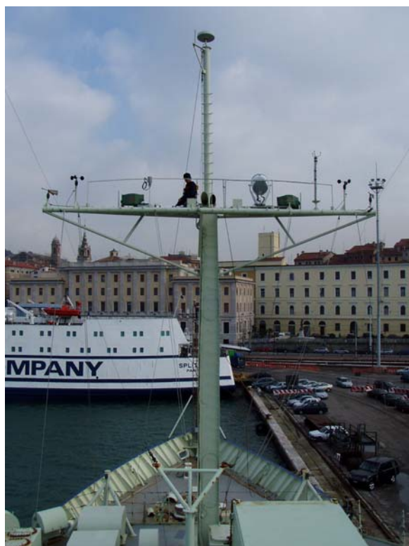
Figure 1. Meteorological sensors on forward mast arm. The sonic wind sensor is the third sensor right side. The cup and vane devices on both ends of the arm belong to the KNORR.
