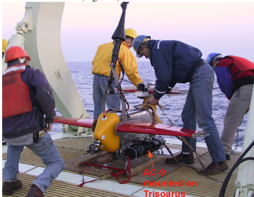
Figure 1. Trisoarus recovered from tow with AC-9 mounted on the lower right side of the vehicle. Other measurements include T, S, dissolved oxygen, beam transmission at 660 nm, chlorophyll and CDOM fluorescence.
