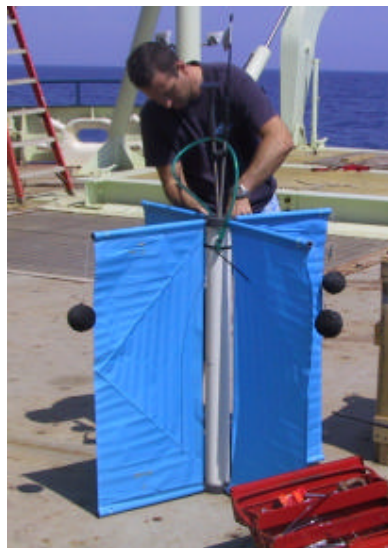
Figure 1. Preparing a CODE-GPS drifter for deployment.
