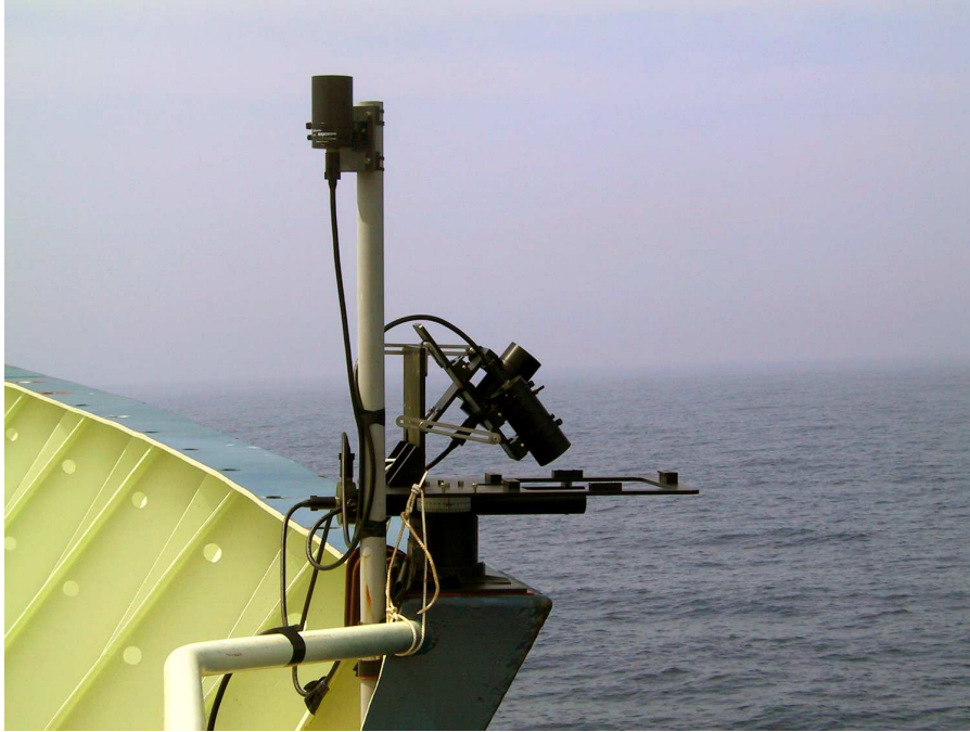
Figure 2. Satlantic MicroSAS system used to continuously measure upwelling radiance and reflectance during daylight.
