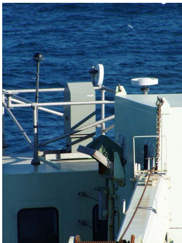
Figure 2. The ceilometer is the 1.2 m high gray, rectangular box on top of an observation cabin.
