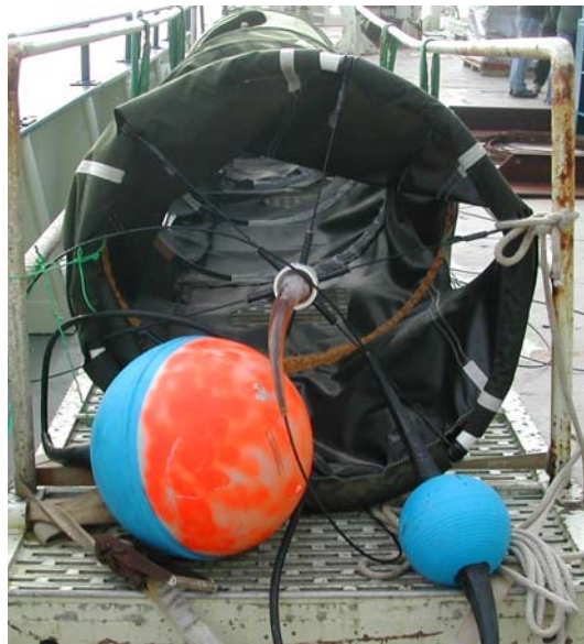
Figure 2. SVP drifter with holey-sock drogue, intermediate float and surface ball.
