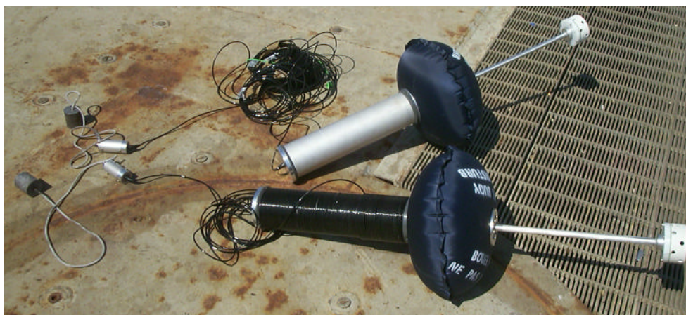
Figure 5. CMOD (XAN-3) drifters with thermistor chains.
