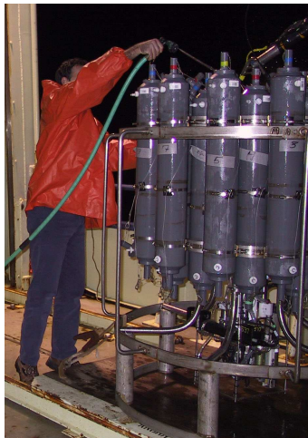
Figure 4. CTD/rosette on deck of ship after recovery from profile.
